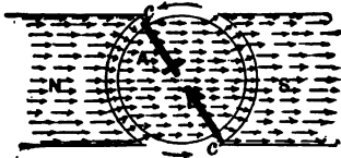
FIG. 204.—ACTIVE CONDUCTOR ENTERING POLAR FLUX.
